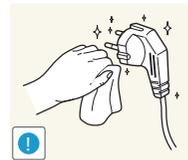
Clean any dust around the pins of the power plug or the power socket with a dry cloth.
