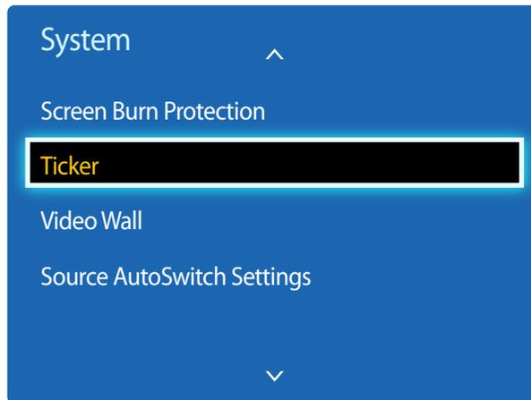
Input text while a video or image is displayed and display the text on the screen.
