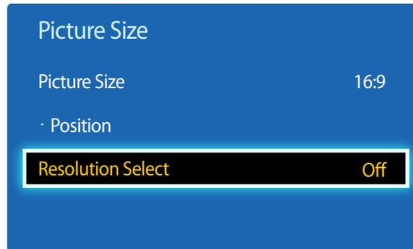
If the picture is not normal even when the resolution of the graphics card is one of the following, you can optimize the picture quality by selecting the same resolution for the product as the PC using this menu.
