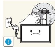
During a lightning or thunderstorm, power off the product and remove the power cable.
