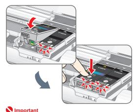
If the front (innermost) part of the ink tank (A) is sticking up, push down on the Canon logo on the ink tank as illustrated below. Do not remove the ink tank forcibly.
