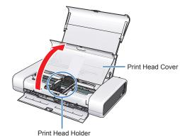
2 Unlock the Print Head Lock Lever by squeezing both tabs inward.
