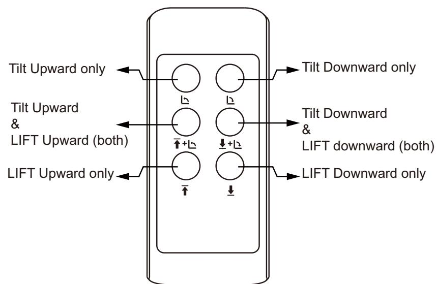
Designated Remote control shall be compatible with specific motorized cart
