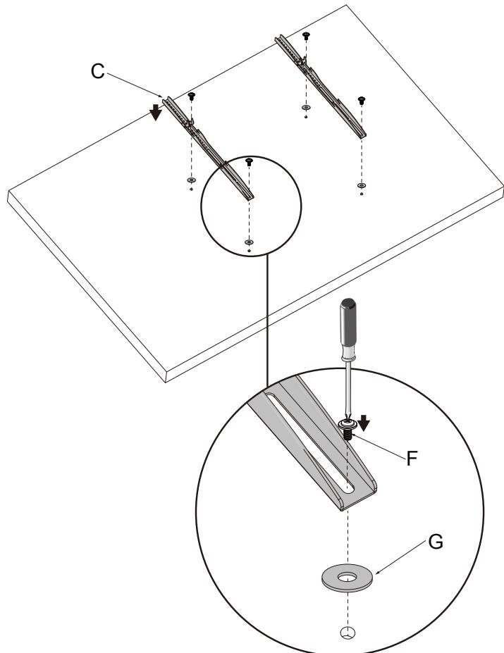
Make sure mount bracket being upright-before display to be installed
