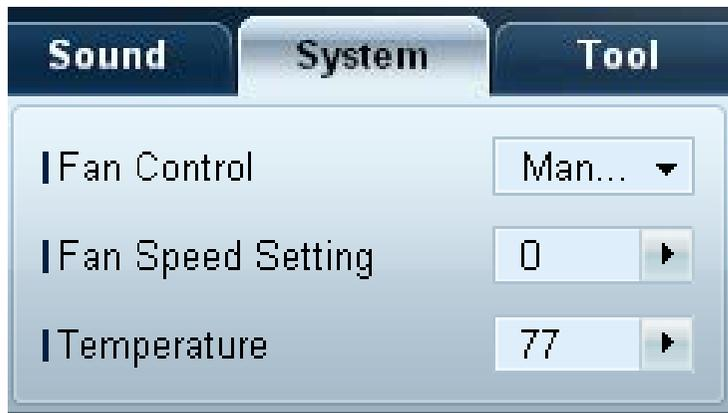
Configure the settings required to detect the fan speed and internal temperature for the product's protection.
