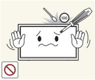
Do not insert metallic objects (chopsticks, coins, hairpins, etc) or objects that burn easily (paper, matches, etc) into the product (via the vent or input/output ports, etc).
