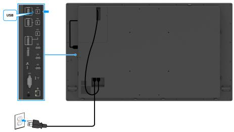
Figure 24. Connecting the USB cable
