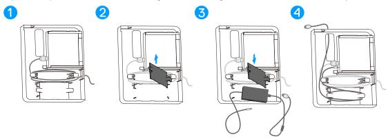
Figure 16. Plug in the power adapter and route the cables
