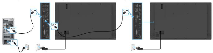
Figure 22. Connecting the monitor for the DisplayPort Multi-Stream Transport (MST) function
