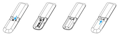
Figure 32. Inserting the batteries in the remote control
