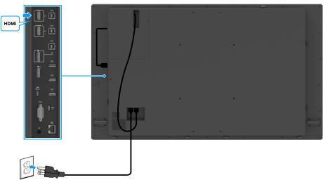
Figure 25. Connecting the HDMI cable
