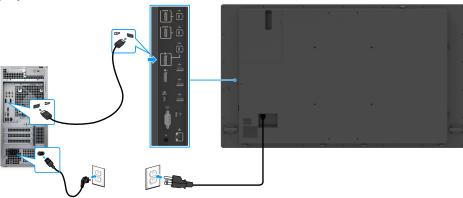
Figure 20. Connecting the DisplayPort cable
