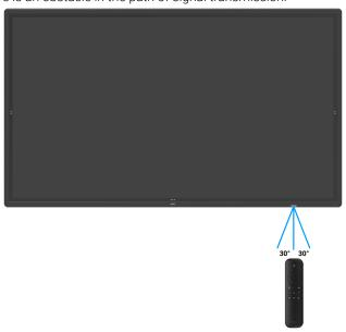
Figure 33. Operating range of the remote control
