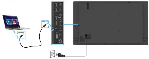
Figure 21. Connecting the USB Type-C cable
