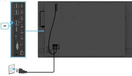
Figure 26. Connecting the DisplayPort cable
