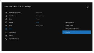
Figure 42. Select the required option to lock
