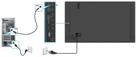
Figure 18. Connecting the USB cable
