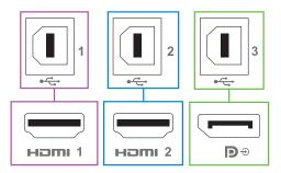
Figure 4. Input sources and USB pairing
