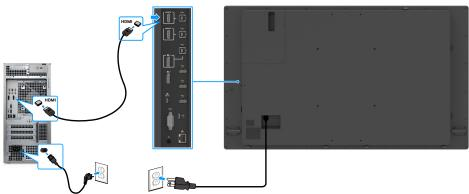
Figure 19. Connecting the HDMI cable
