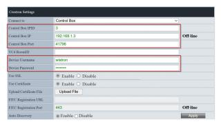
Figure 69. Connection to Control Box
