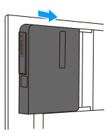
Figure 17. Slide the OptiPlex holder back into the monitor
